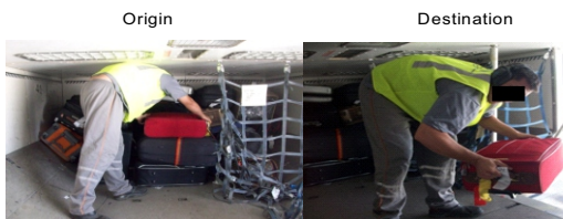
Figure 4: Removing the bags and placing them at the entrance of the cargo hold of the aircraft
