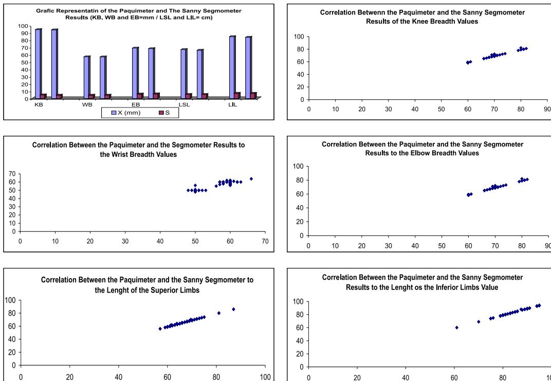
Little differences regarding the results of the measures carried out the three examiners were found between the paquimeter and Sanny segmometer when these measurements were compared. The differences between E1 and E2 to KB, WB, EB, LSL, LIL are 3,58%, 5,48%, 5,48%, 5,85% e 4,76%, between E1 and E3 are 1,40%, 1,87%, 2,42%, 2,66% e 2,26% and between E2 and E3 are 2,09%, 3,40%, 2,85%, 2,94% e 2,33%.
