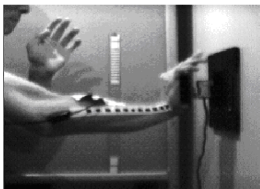
Fig. 3. Impact image taken by the High Speed Camera. The color contrasts in the forearm indicate the markers used in the analyses. The color contrasts in the ruler were used to determinate the conversion scale from pixels to centimeters.
