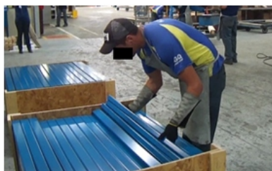
Figure 10 - Storage of the painted parts
