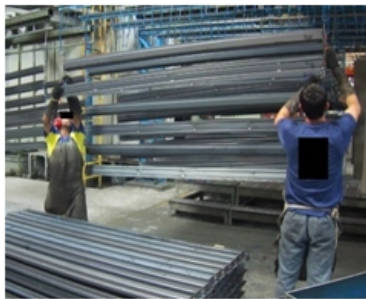
Figure 6 - To hang the pieces on the hooks
