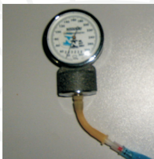
Figure 1: Pressure gauge adapted to the end of an infusion set to verify the cuff pressure.
