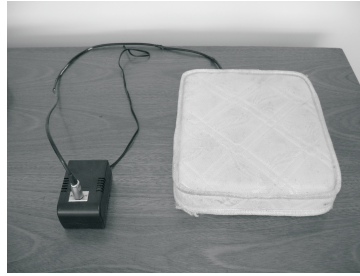
Figure – mattress with the electromagnetic field, adapted to the size of the animals cage.
